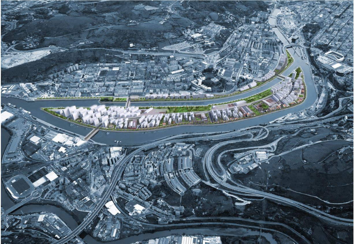
Figure 19. Computer graphics impression of the adaptation measure studied in the Bilbao case. The new development of the Zorrotzaurre district of Bilbao by its conversion from a peninsula into an island, by means of opening a 75 m wide channel. Source: Saitec (2007).
